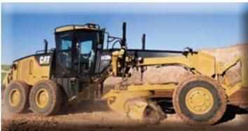
4. This is **not** an Articulating Trac Hoe with a true brush, it is a **Motor Grader** which is used for grading in construction projects.
