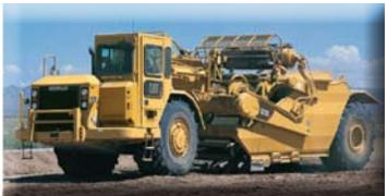
2. This is **not** a Bulldozer! It is actually a **Wheel Tractor Scraper** which is used for earth moving in large construction projects. The back section is called the bowl & can be lowered to cut soil & materials.
