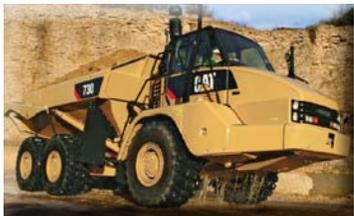
3. This is actually a “dump truck” but it is correctly called an **Articulating Truck** because of its drive system. This is a big truck and is great for off road rough terrain.
