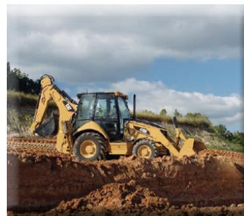
7. This is a **Backhoe** and it is used to move materials in construction, to push materials and to dig. It can also be used to move snow.
