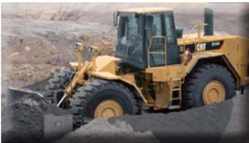
1. While this can be an Earth-mover it is technically a **Cat 824 Wheel Dozer**. It is used for moving soil, stone, trash and other materials.
