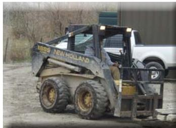
6. This is **not** a Bobcat which is actually a brand name. It would be the same as calling a soft drink a Coke. It is a **New Holland Skid Steer** which is used to move materials and can have any number of implement attachments.
